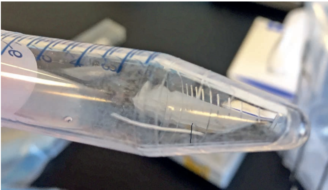
Image 1. Picture of the cracked centrifuge tube from Case 1.
