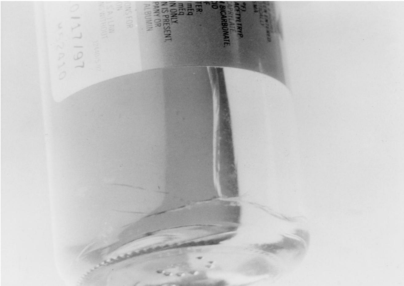
**Figure 2.** Albuminar vial with large crack. Four (1.5%) of the 276 Albuminar vials examined at the FDA had readily visible cracks measuring  $\geq 6$  mm, as seen here.
