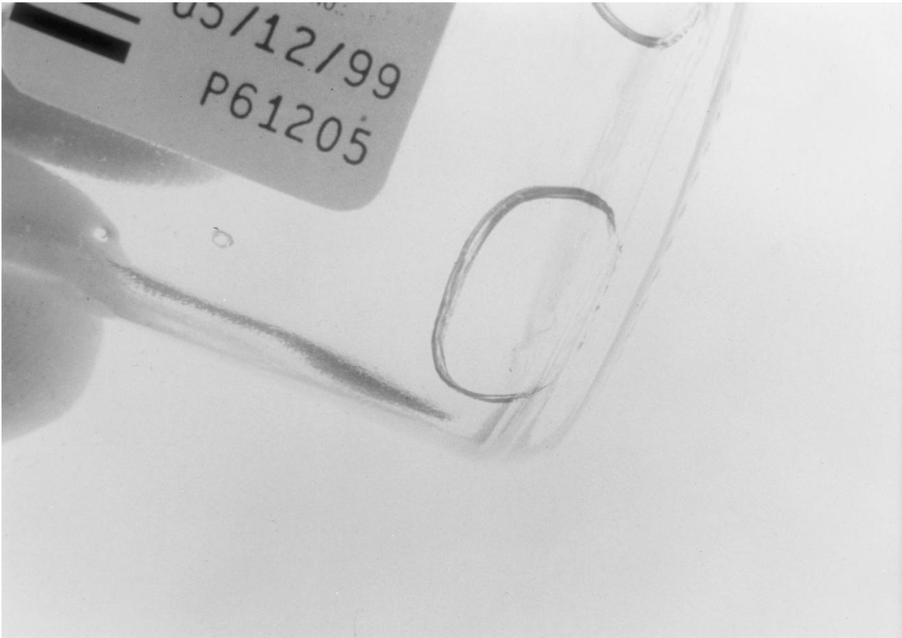
**Figure 1.** Albuminar vial with small crack. Of 276 Albuminar vials examined at the FDA, 152 (55%) had chips, dents, or scratches measuring 1–5 mm, as seen here.
